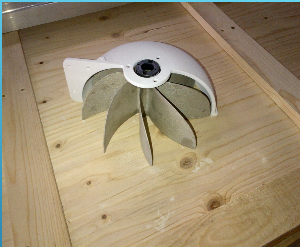
Second Prototype Created on 3D Metal Printer NS Community College, Dartmouth Campus
