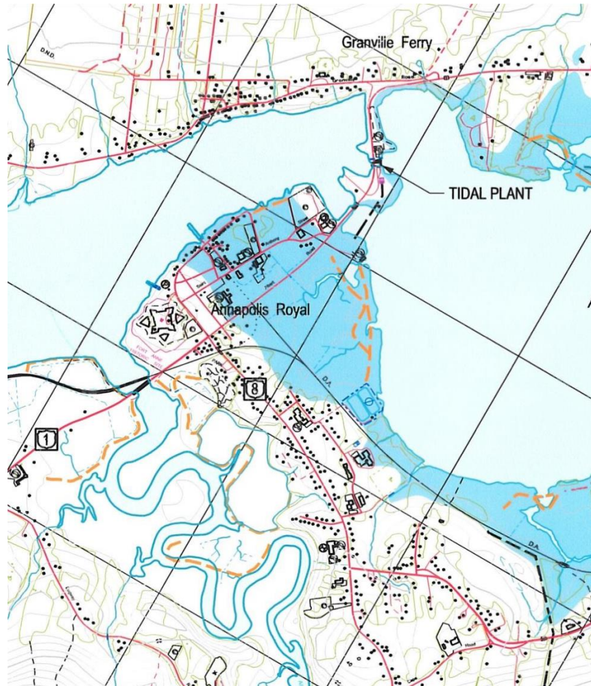
Probable Maximum Flood Inundation Limits (Source: Nova Scotia Power, Emergency Preparedness Plan Paradise Hydro System, MCCAP p.1)
