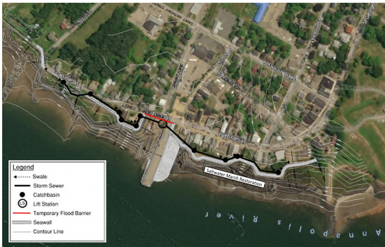
Figure 3-1: Schematic of Proposed Seawall
