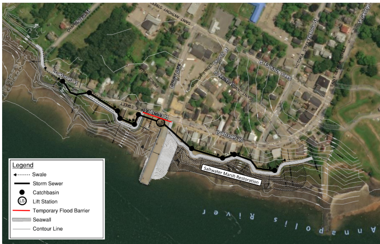
Figure 3-1: Schematic of Proposed Seawall
